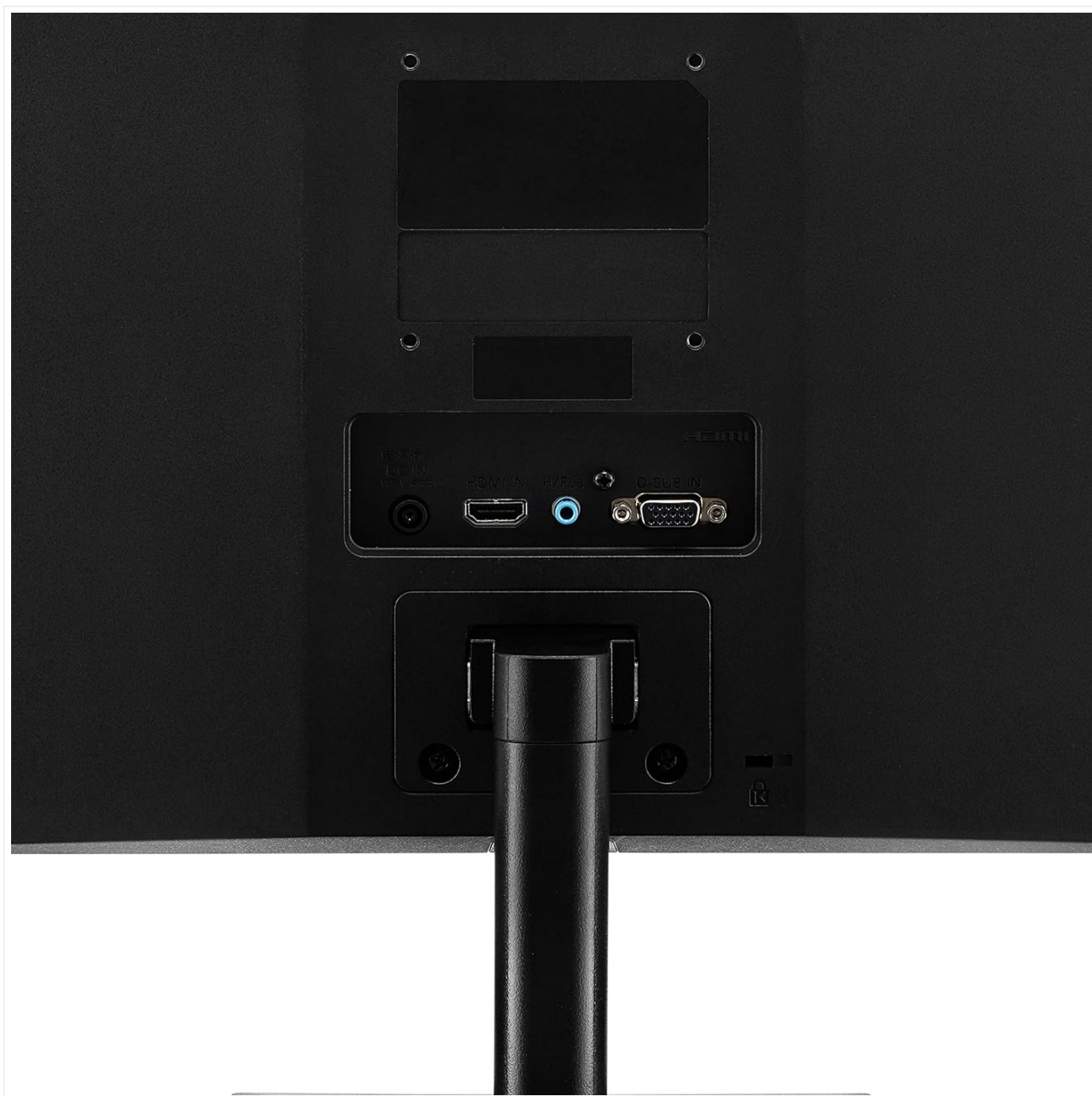
Image: Close-up view of the monitor's rear input/output ports. From left to right, these include the power input, HDMI port, headphone out jack, and D-Sub (VGA) port.
