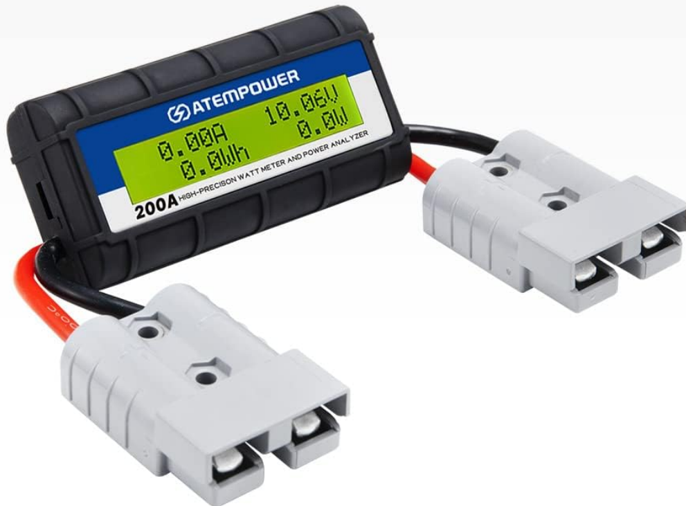
Figure 5.4: Measuring the charging rate and total charge from solar panels.
