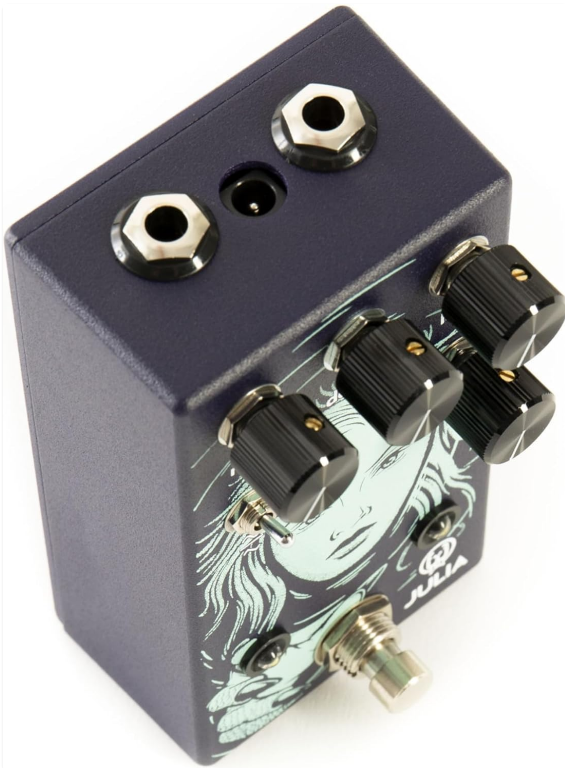
Figure 2: Top view of the pedal, illustrating the input and output jack placement.
