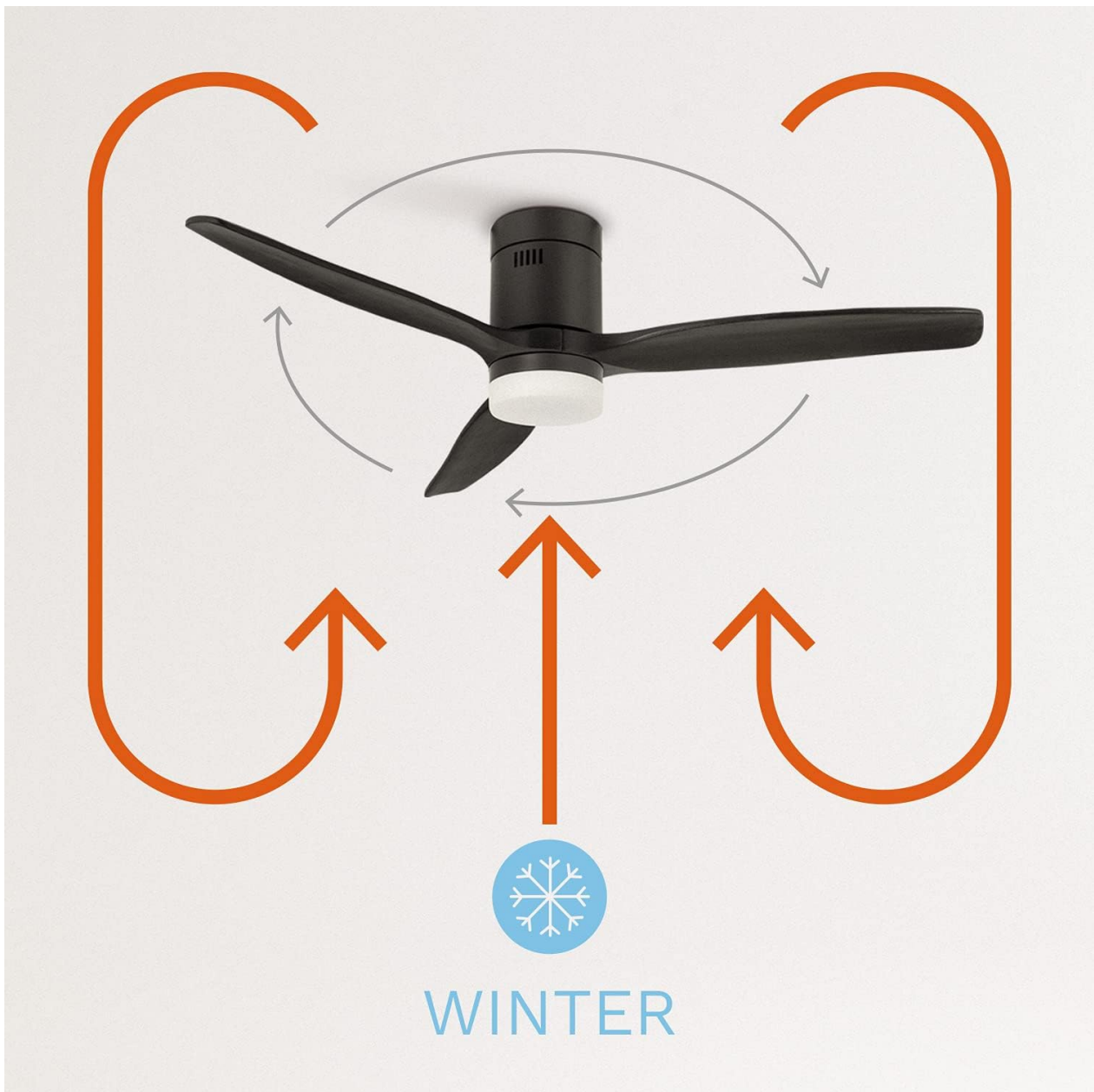
Image 5.3: Winter mode operation, circulating warm air upwards to redistribute heat.
