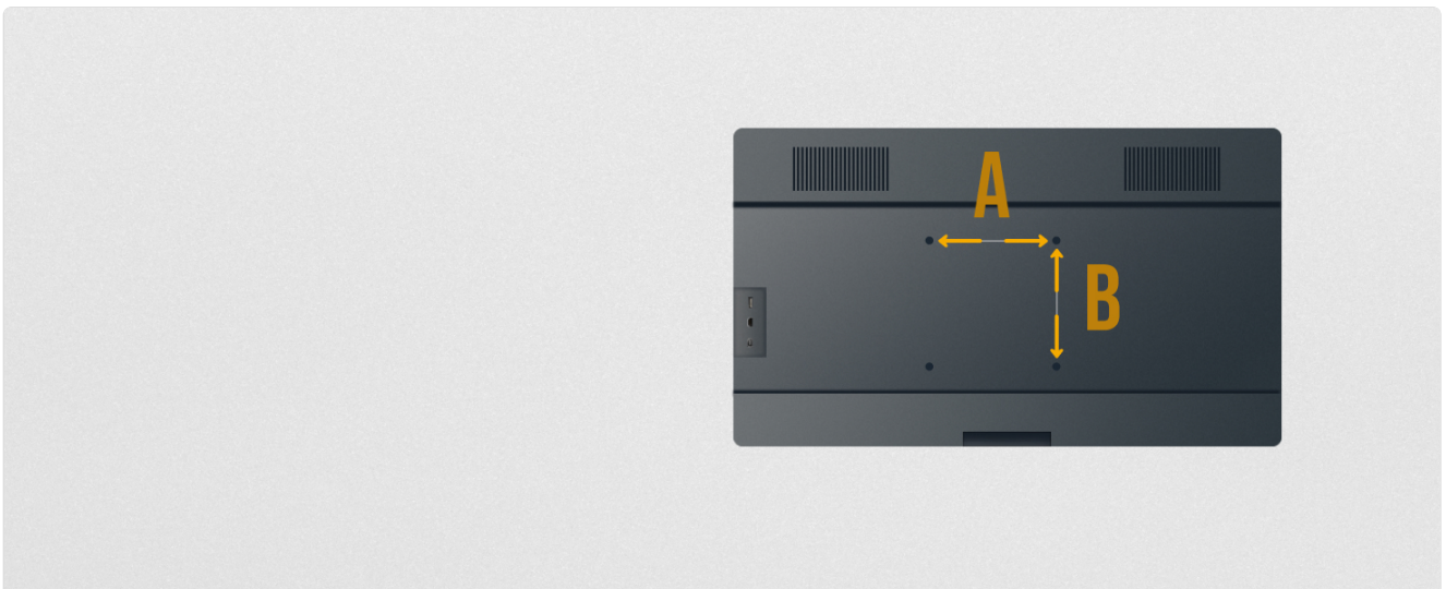
Image: Diagram indicating VESA mounting hole measurements (A and B) on the back of a monitor.
