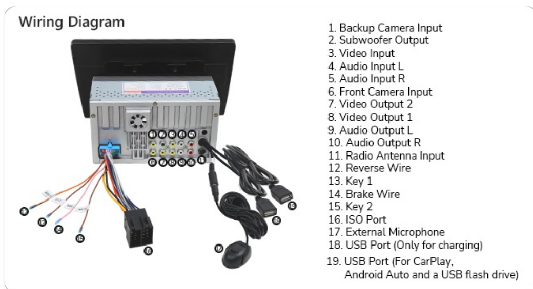
Figure 2.6: Simplified wiring diagram showing key connections like ISO port and USB ports.
