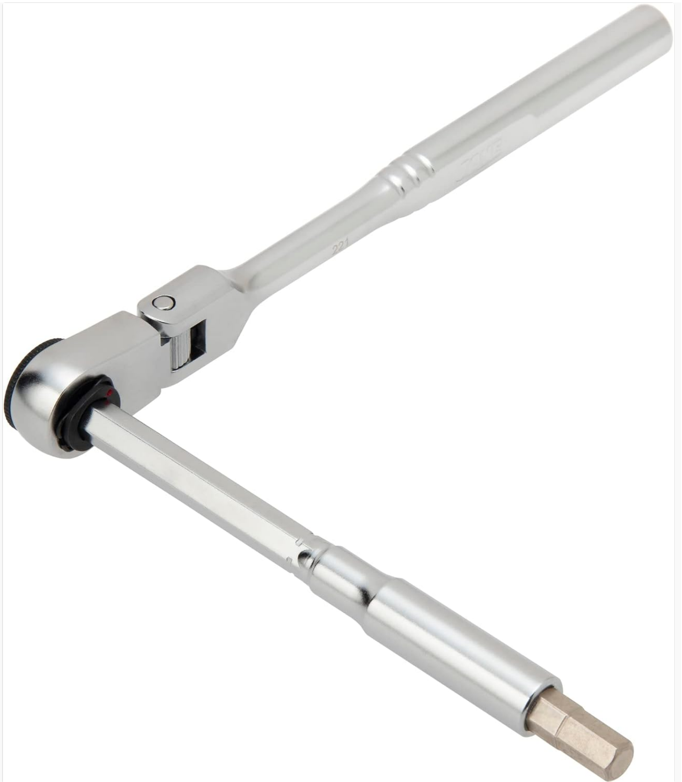
Image 6.1: The ratchet handle and extension bar assembled into a T-handle configuration.
