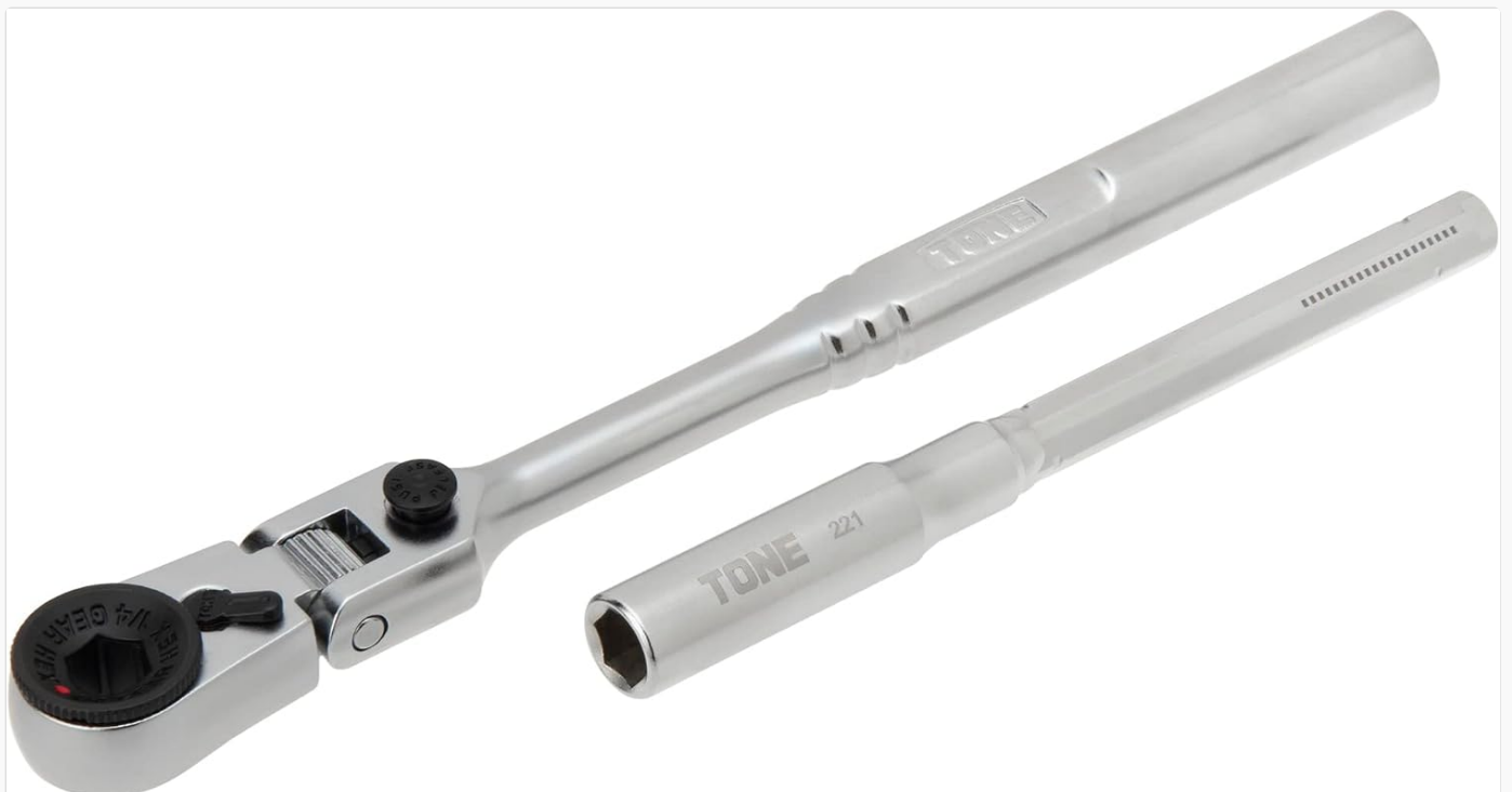
Image 5.1: A selected bit securely inserted into the ratchet handle.
