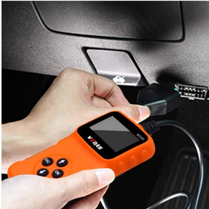
Figure 4: Illustration of the OBD2 port and connector.
