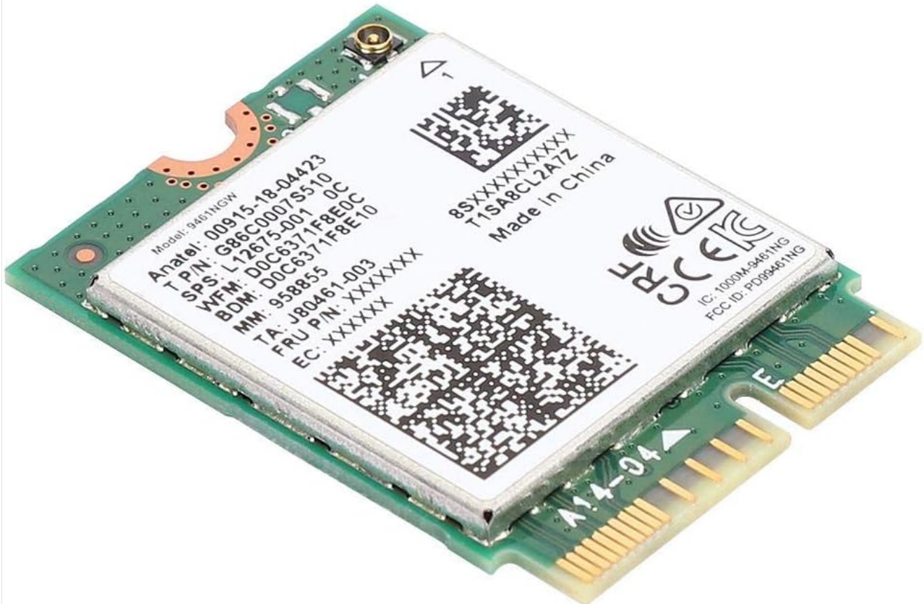
Figure 3.1: The network card supports both 2.4G and 5G wireless networks for flexible connectivity options.
