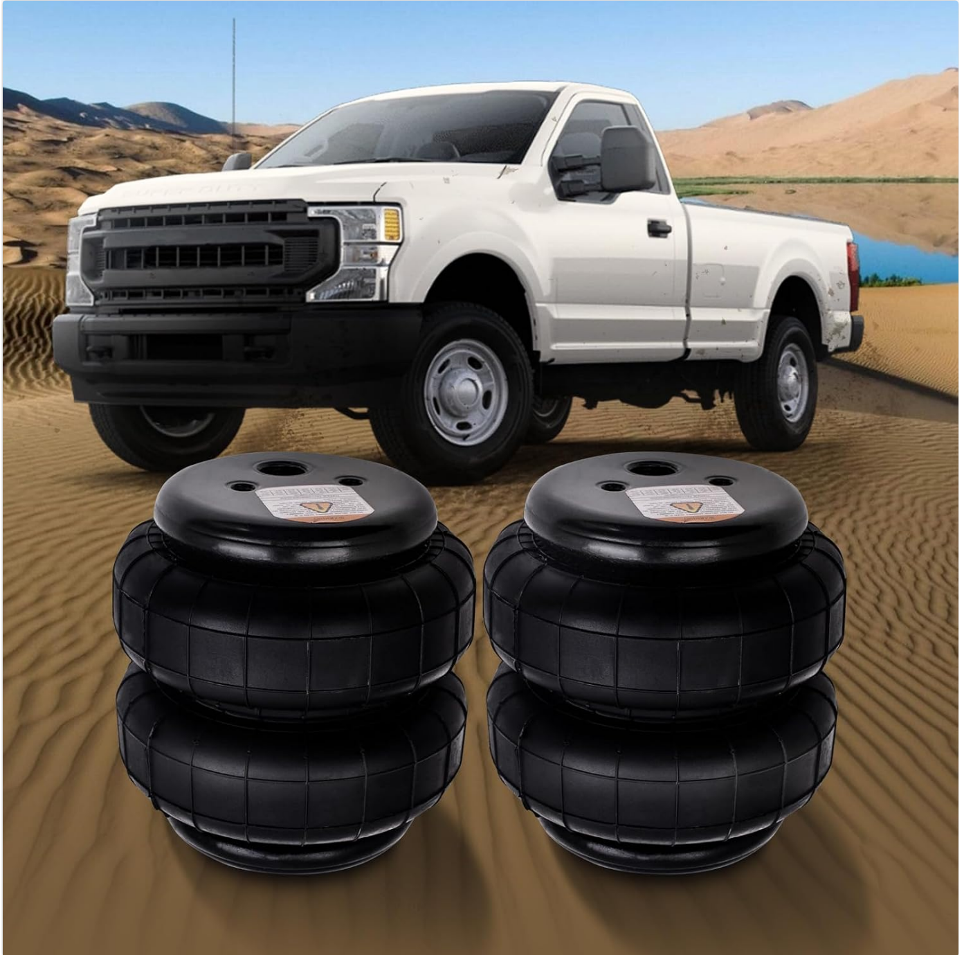
Figure 4.1: Example of a truck equipped with air suspension bags, illustrating how they help maintain vehicle level.
