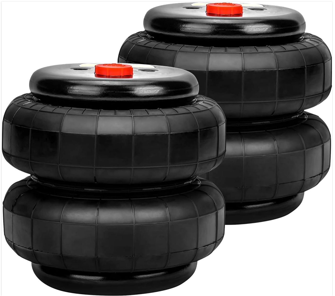
Figure 2.1: Two maXpeedingrods 2500 lbs air suspension bellow bags, showing their compact, robust design.
