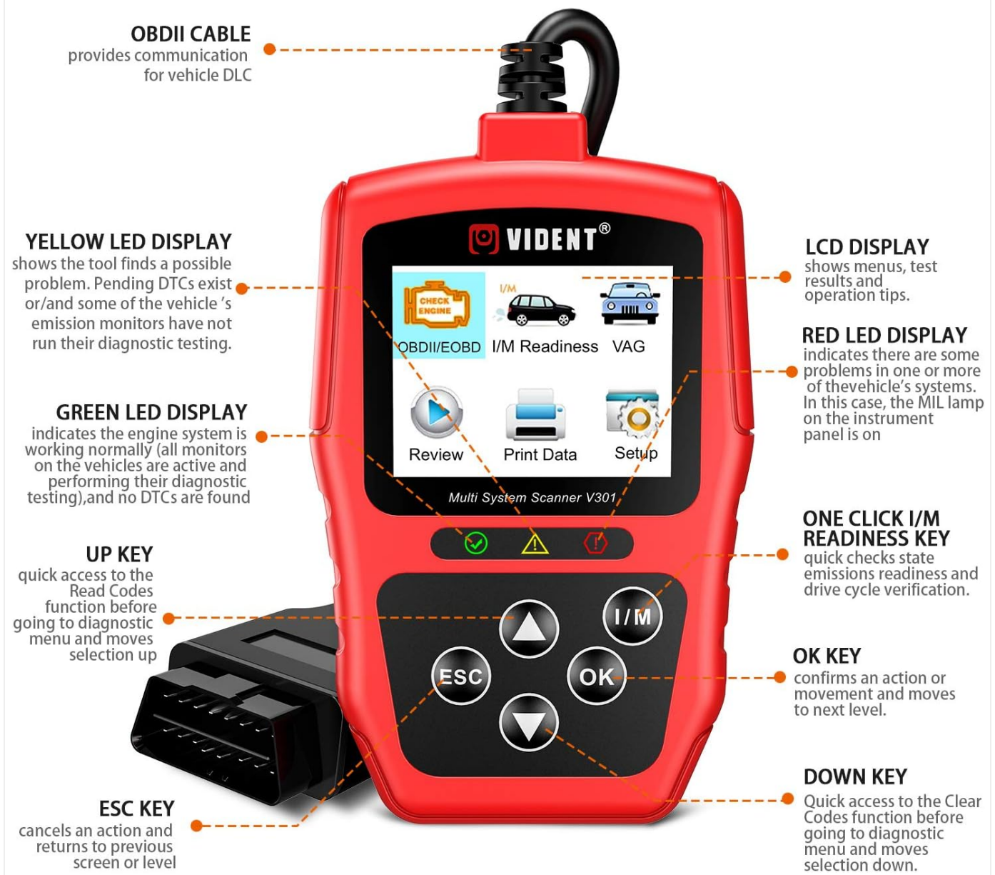
Figure 2.2: Tool Descriptions. This diagram labels the various parts of the V301 scanner, including the OBDII cable, LCD display, LED indicators (Yellow, Green, Red), and control keys (UP, DOWN, ESC, OK, I/M Hotkey).
