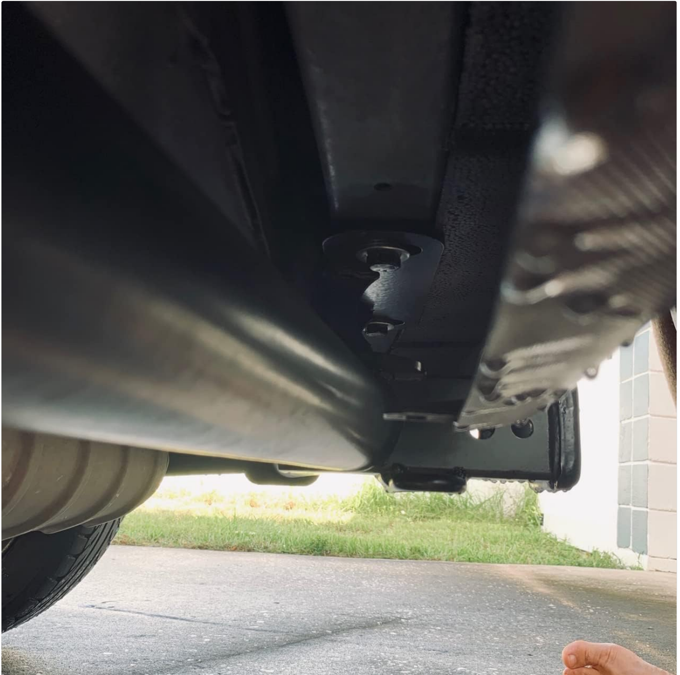
Figure 5.2: Close-up of the hitch attachment points under the vehicle.
