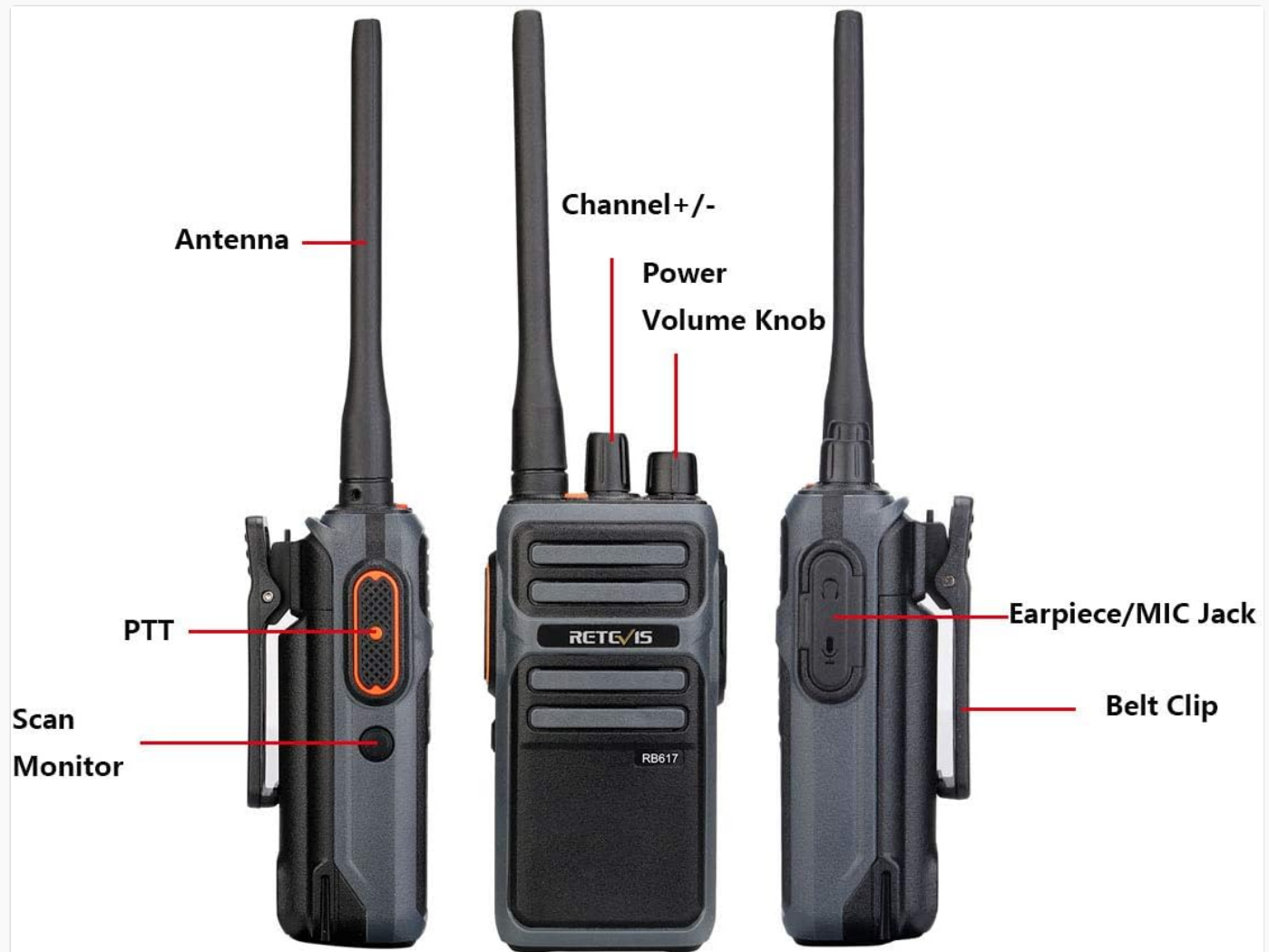
Figure 2: RB617 Component Diagram
