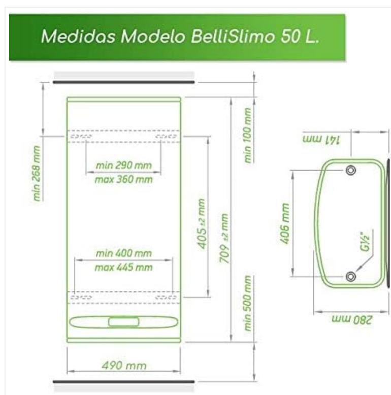
Figure 4: Detailed technical drawing providing all necessary dimensions for the BelliSlimo 50L model, crucial for installation planning.
