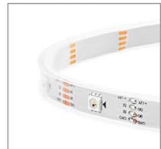
Image 4.4: Illustration demonstrating where to safely cut the LED strip using scissors, indicating that the rest of the strip will continue to function.
