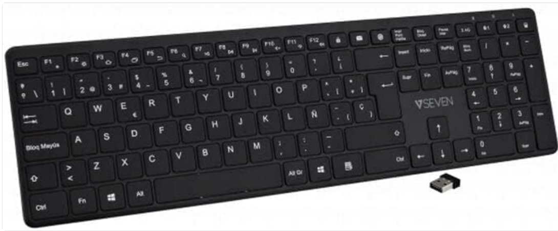
Image: The V7 KW550ESBT keyboard shown with its accompanying 2.4 GHz USB receiver, ready for connection.
