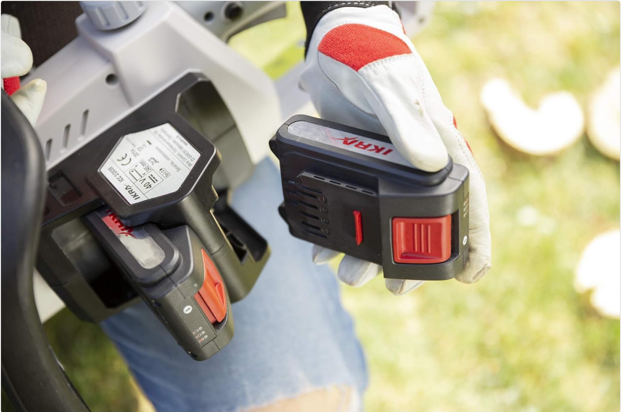
Image: Inserting the battery into the chainsaw.
