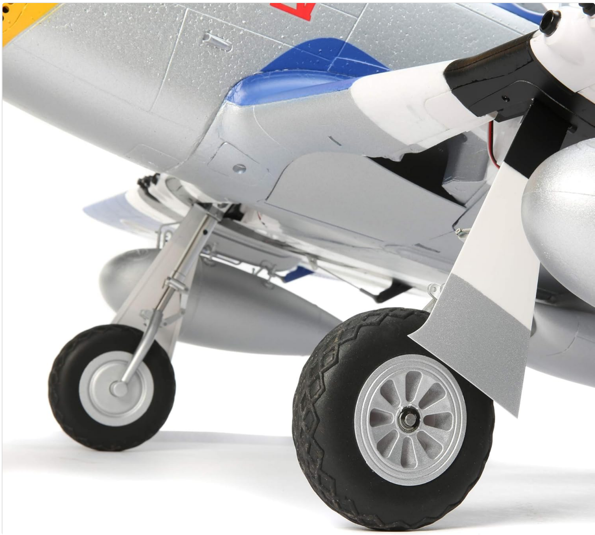
Image: Close-up of the E-flite P-51D Mustang's retractable landing gear with shock-absorbing struts.
