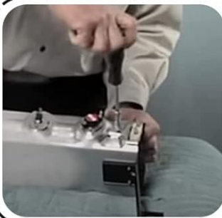
Figure 2: Installation steps for the heating element. This image illustrates the four key steps: inserting the heating wire, fixing the plug, securing with screws, and completing the installation.
