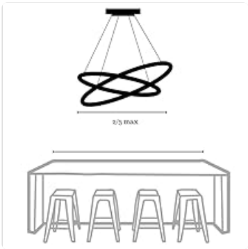
Figure 4: Linear pendant placement over an island. The fixture
