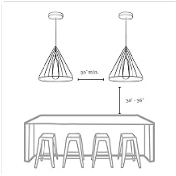
Figure 5: Multiple pendant placement over an island. Maintain 30-inch minimum spacing between fixtures and 30-36 inches above the surface.
