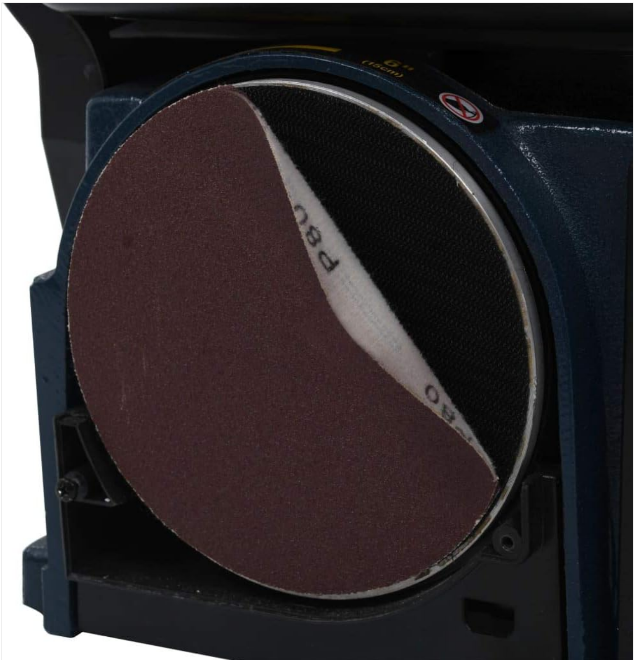
Figure 3.7: A close-up of the sanding disc, showing the adhesive backing for attaching sanding paper (P80 grit shown).
