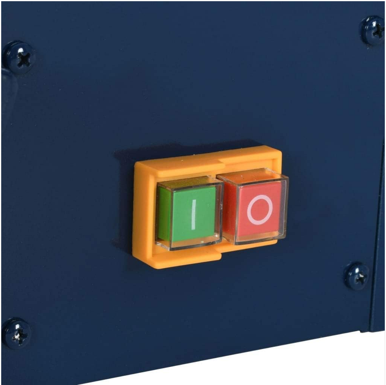
Figure 3.6: The main power switch, featuring a green 'I' button for ON and a red 'O' button for OFF.
