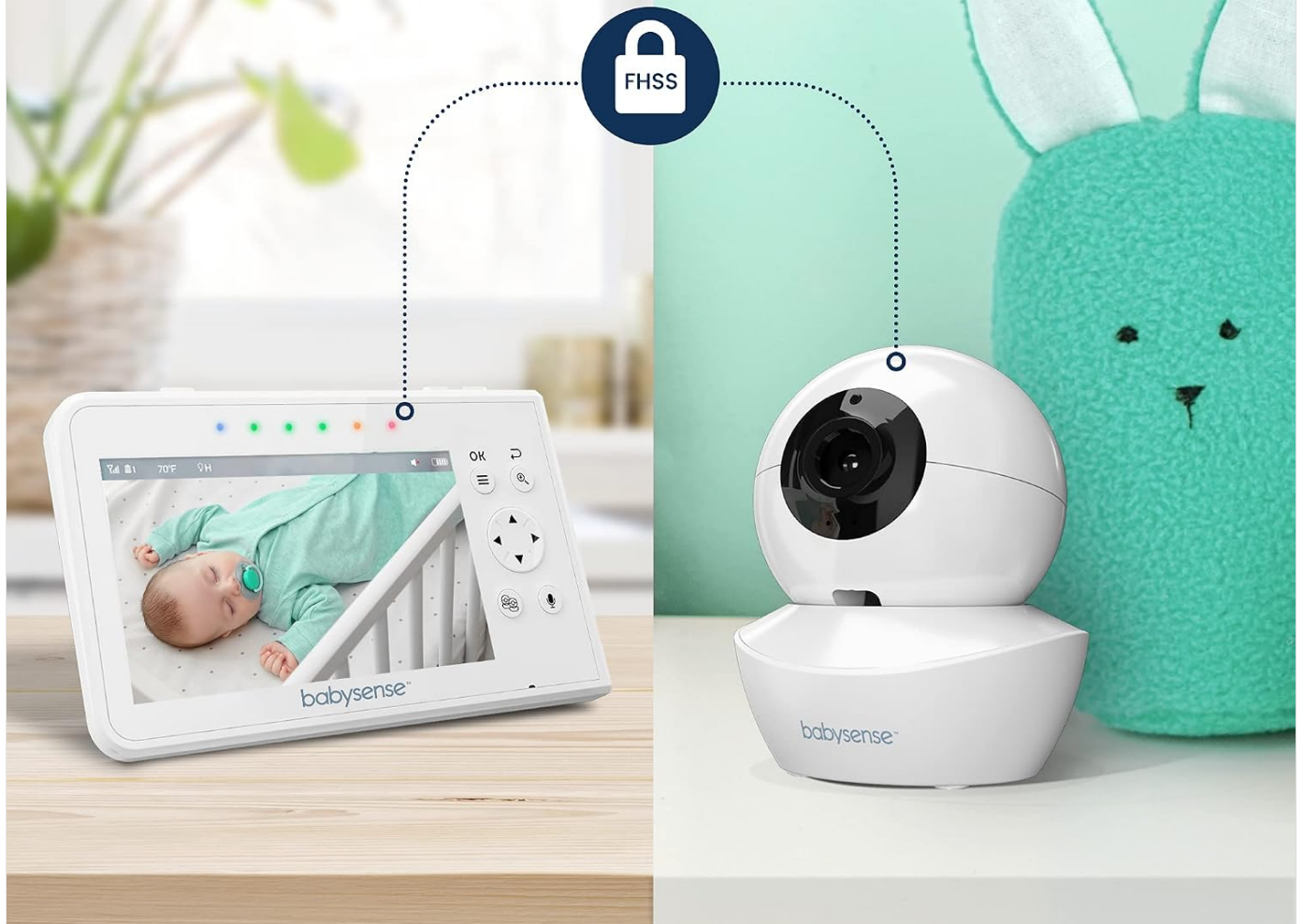
Figure 3.3: The monitor utilizes 2.4GHz FHSS Technology for a secure and hack-proof connection.
