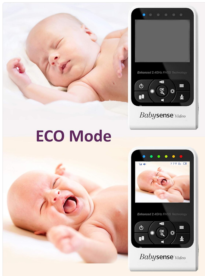
Figure 2: The Parent Unit display shows the live video feed from the baby unit. Control buttons below the screen allow for various functions including power, volume, brightness, talk-back, and menu access. The top of the unit features LED indicators for signal strength and battery level.
