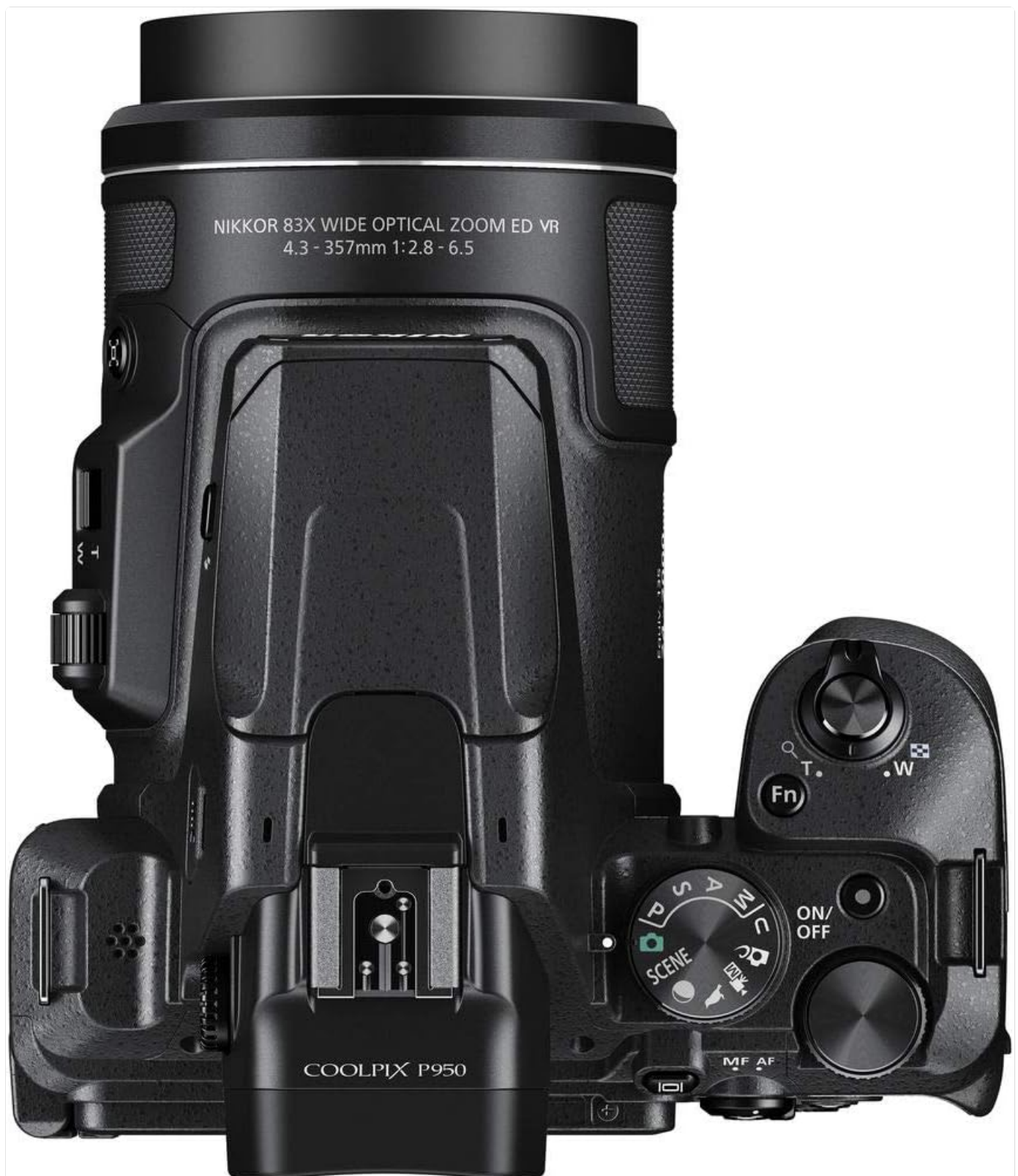
Figure 2.1: Top view of the Nikon COOLPIX P950, showing the ON/OFF button and mode dial.
