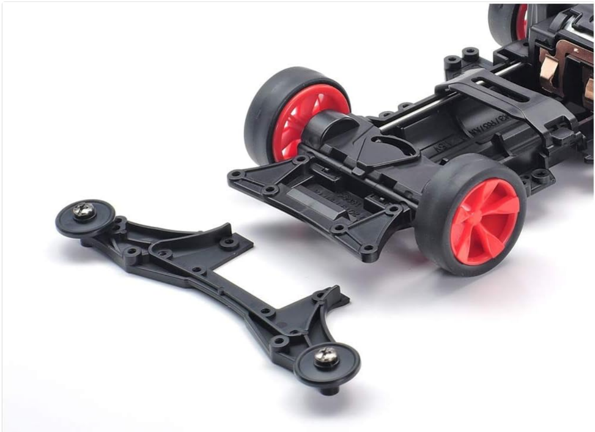
Image: The front bumper/roller stay shown detached from the main chassis, ready for assembly.
