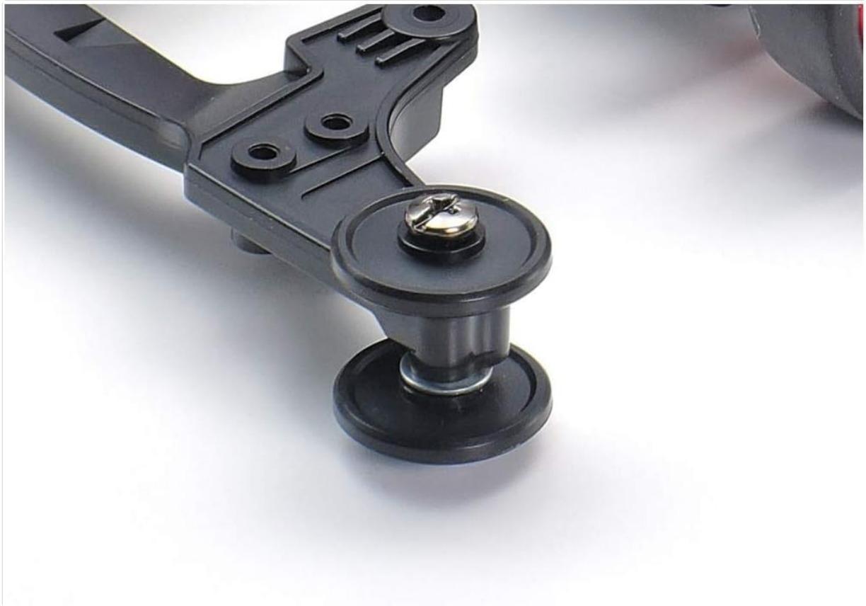
Image: A close-up of a roller attached to the bumper stay, demonstrating its function for track guidance.
