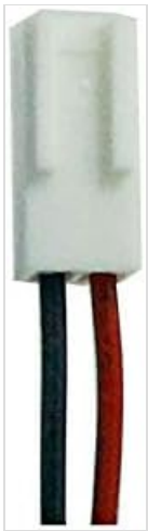
Image 3: Close-up view of the battery's connector. This image highlights the two-pin white connector with red and black wires, used for connecting the battery to the device or charger.
