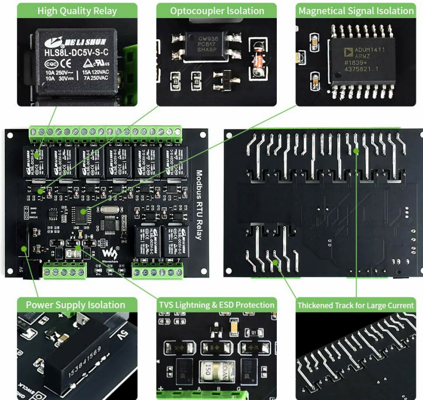
Image 3.1: This image provides a detailed view of the module's internal components, highlighting the high-quality relays, optocoupler isolation, magnetic signal isolation, power supply isolation, TVS lightning & ESD protection, and thickened tracks for large current.
