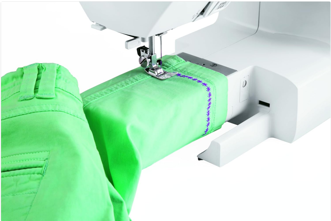
Image 6.2: The Usha Janome Marvella sewing machine demonstrating its free arm capability by stitching the hem of a green pant leg. The accessory box has been removed, allowing the fabric to fit around the narrow arm for easier sewing of cylindrical items.
