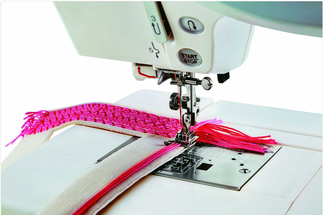
Image 6.1: A close-up view of the sewing machine needle and presser foot in action, demonstrating a decorative stitch being applied to a piece of fabric with fringe. This illustrates the machine's capability for various stitch patterns.
