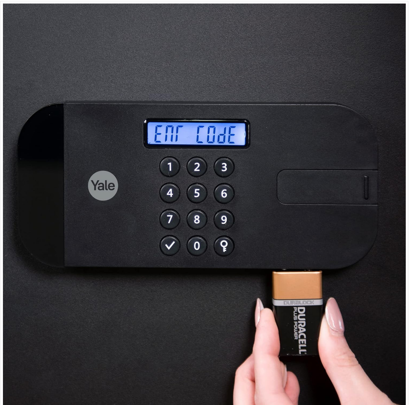
Figure 4.4: A close-up demonstrating how to apply a 9V battery to the external power terminals for emergency access when internal batteries are dead.
