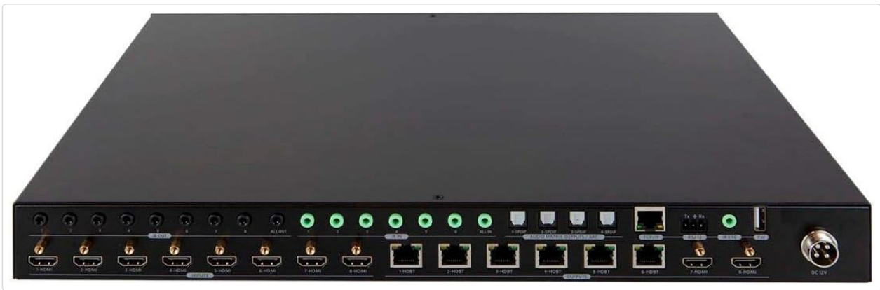
Figure 2: Matrix Unit Rear Panel. This image shows the comprehensive rear panel of the matrix, featuring eight HDMI input ports, seven HDBaseT output ports, one local HDMI output, various audio breakout ports (SPDIF, RCA), an Ethernet port for control, an RS-232 port, and the DC power input.
