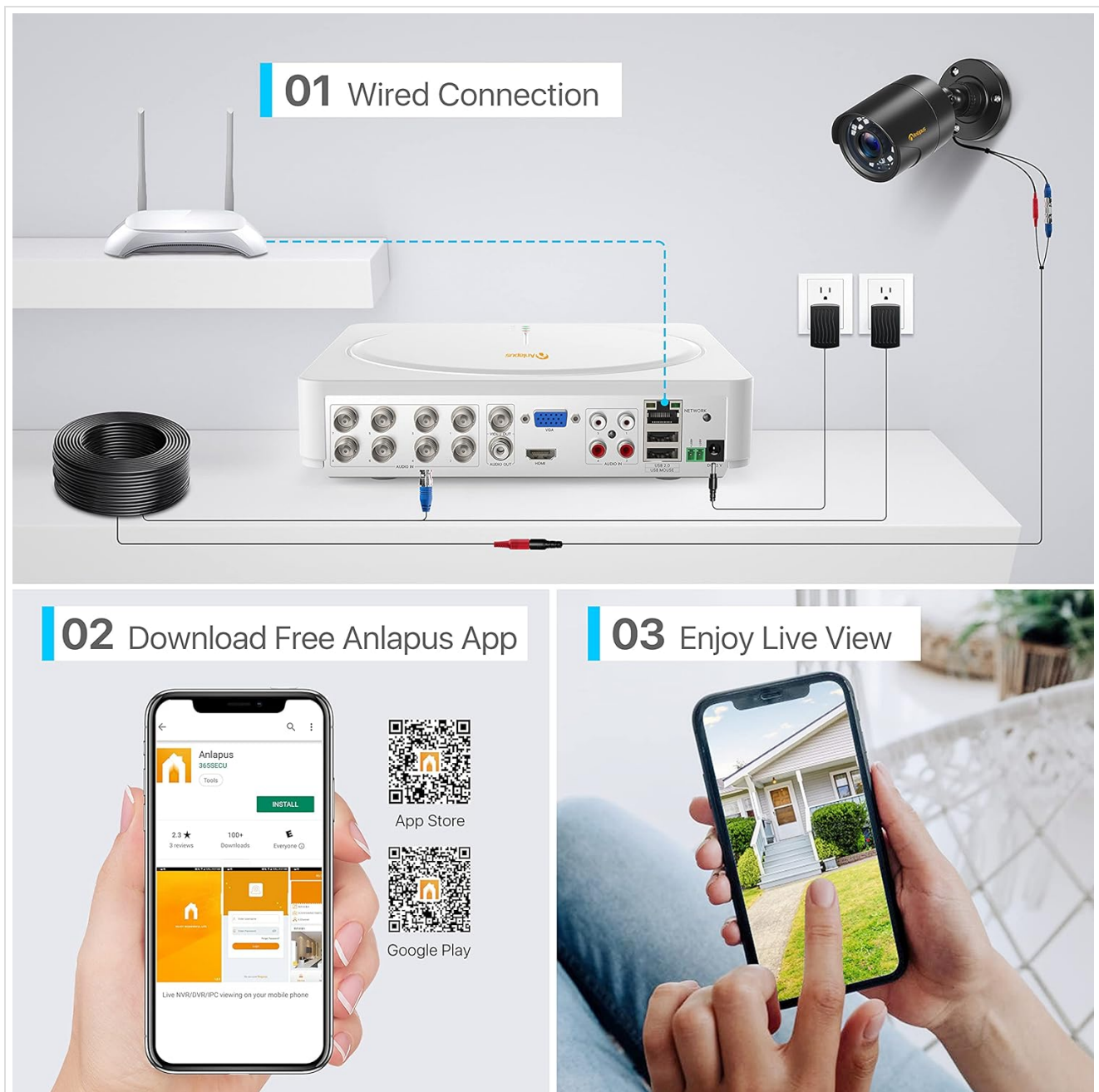
Figure 3.2: Visual guide for connecting cameras, power, mouse, monitor, and network cable to the DVR.
