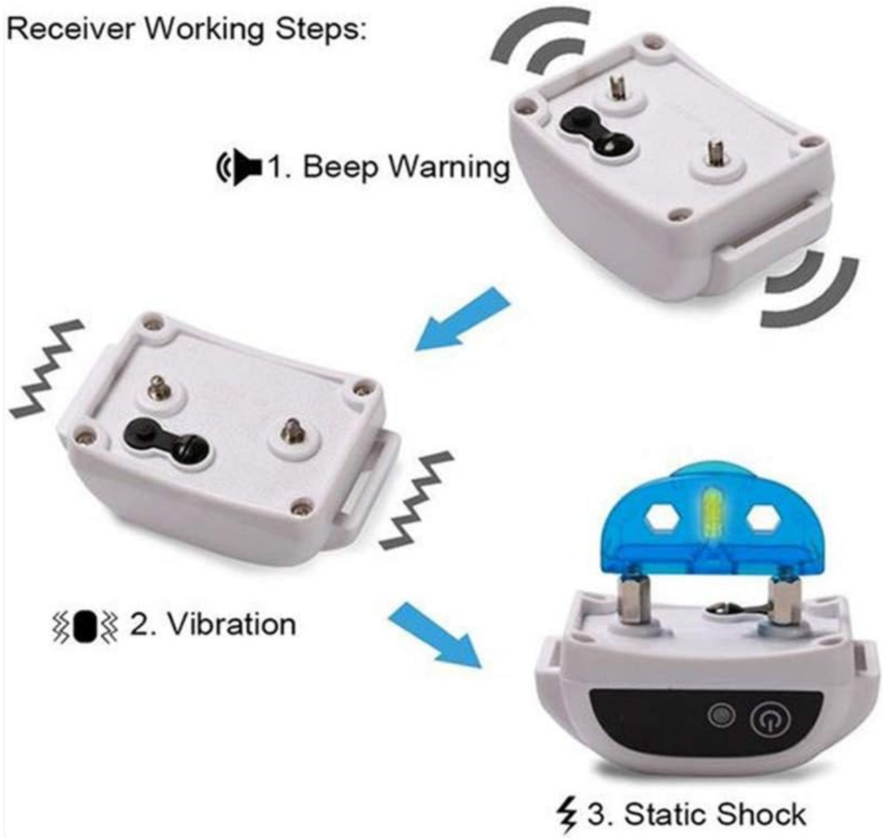
Figure 5.1: The three-step correction process of the receiver: 1. Beep Warning, 2. Vibration (implied by progressive stimulation), and 3. Static Shock.
