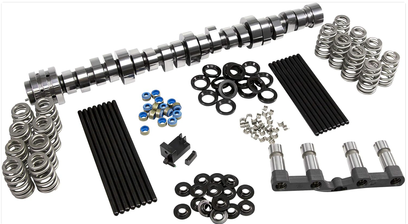
Image 1: Overview of the Comp Cams Master Cam Kit components. This image displays the camshaft, a set of valve springs, pushrods, lifters, and various smaller components such as retainers and valve locks, which are typically included in a comprehensive cam kit.
