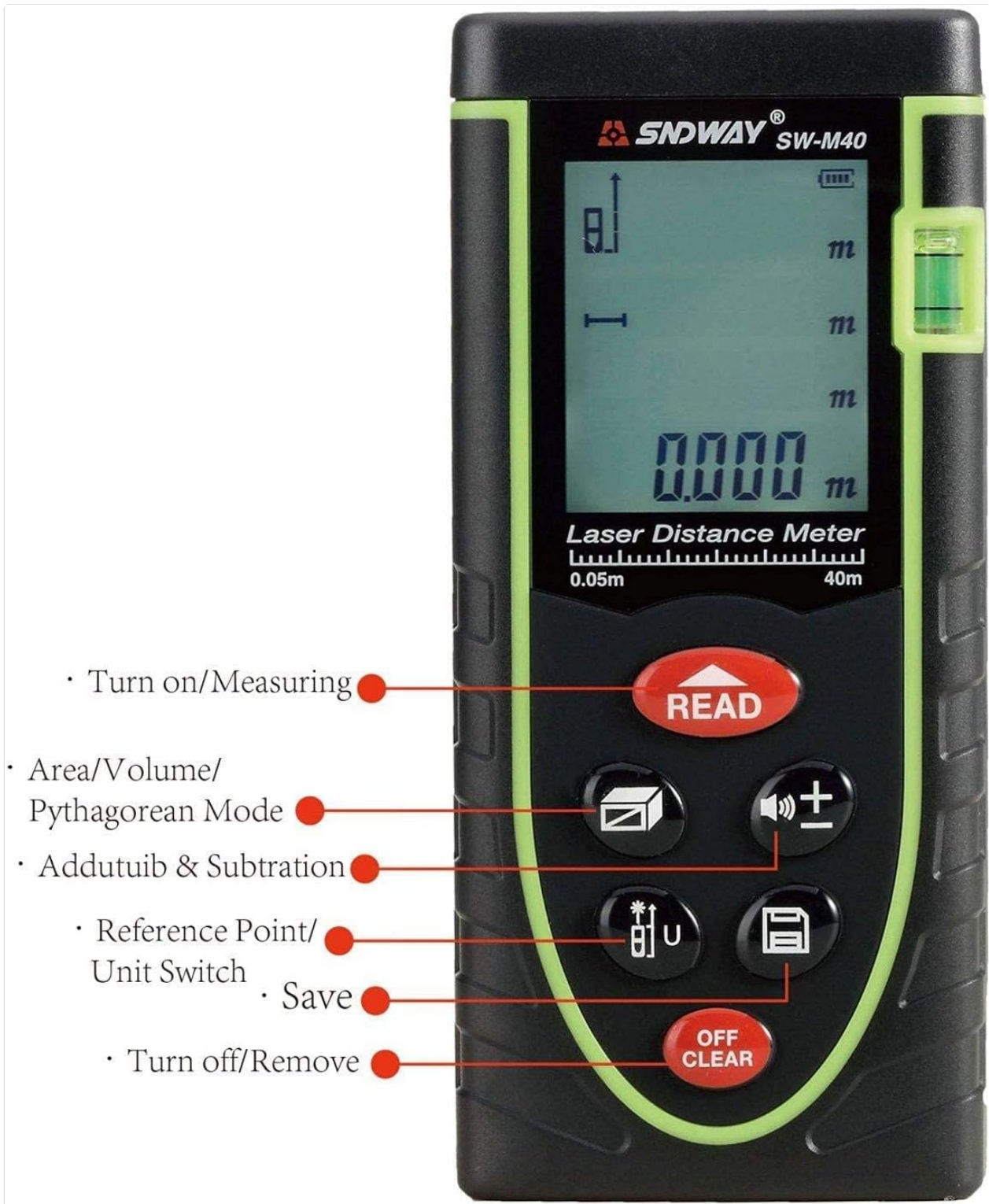
Figure 3.3: Control panel with button functions.
