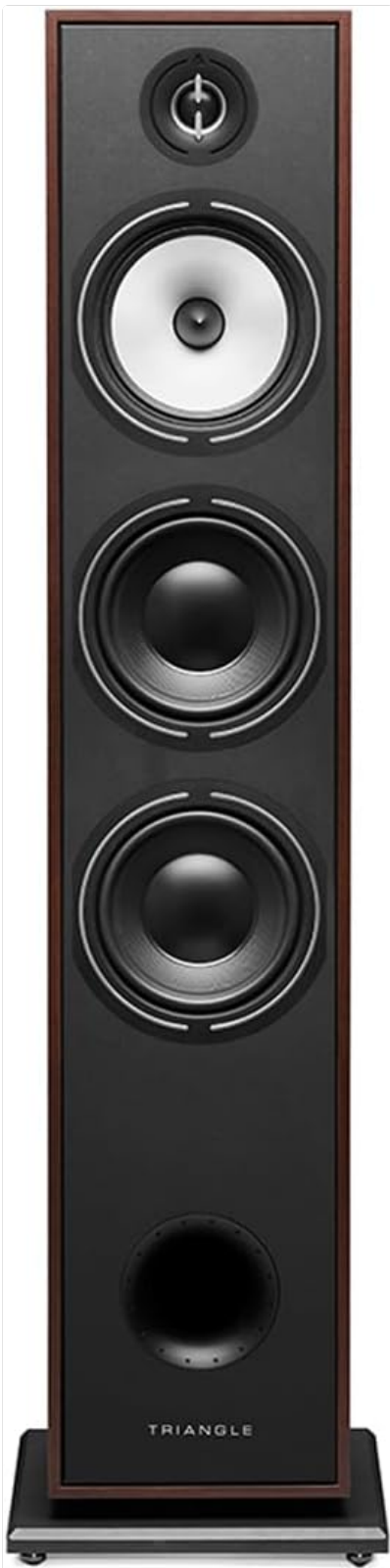
Figure 4.2: Front view of the BOREA BR08, showcasing the 25mm EFS silk dome tweeter, 16cm cellulose paper midrange, and two 16cm fiberglass bass drivers.
