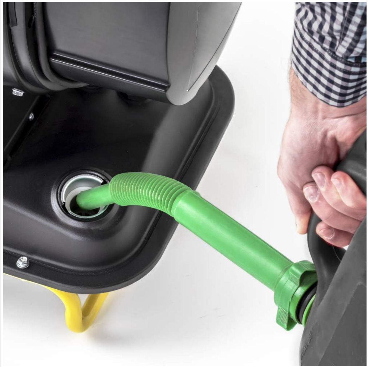
Figure 3.1: Fueling the TROTEC IRO 15 heater. Use a funnel to prevent spills.
