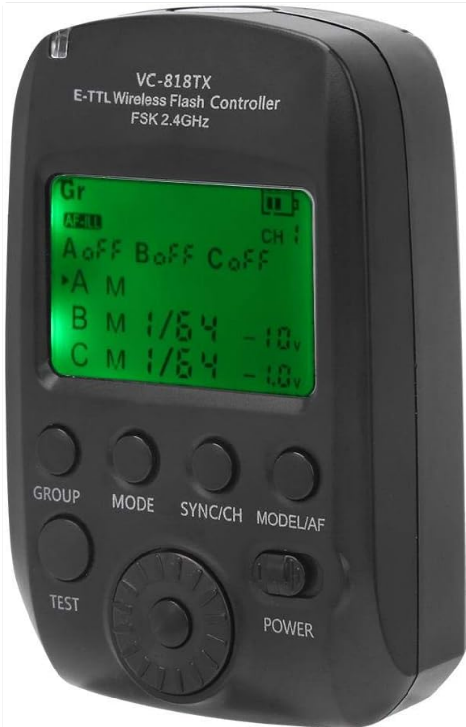
Image 3.1: Front view of the VC-818TX controller, highlighting the LCD display, GROUP, MODE, SYNC/CH, MODEL/AF, TEST, and POWER buttons, and the control dial.
