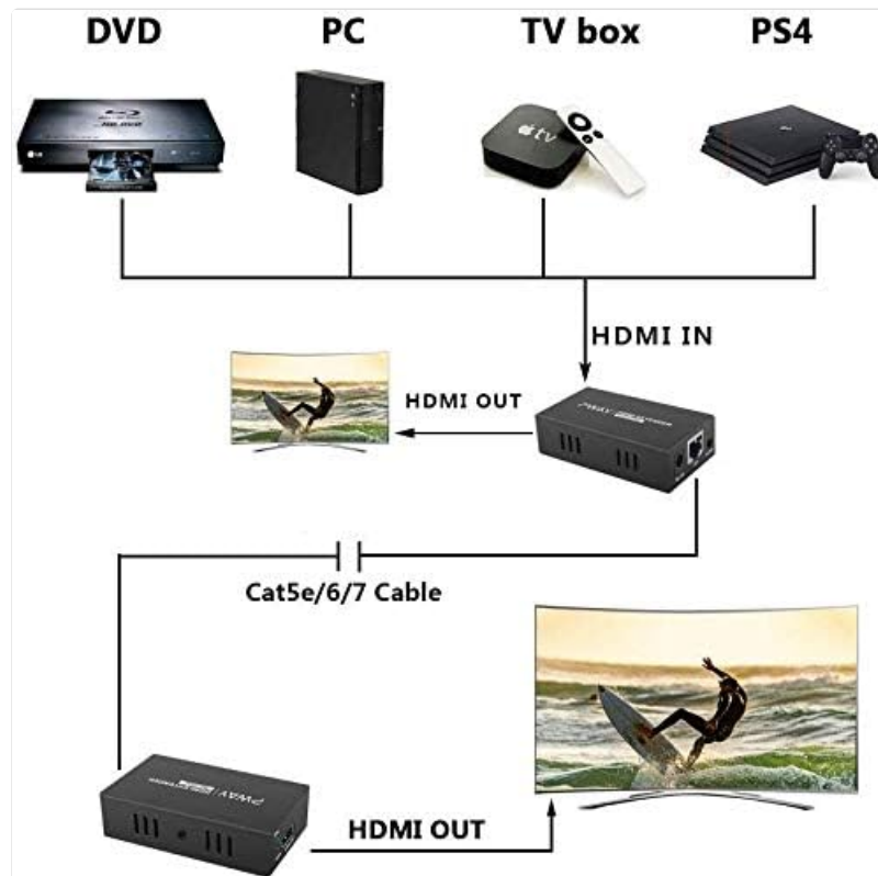
This diagram illustrates the typical connection setup, showing how to connect the HDMI source, transmitter, Cat5e/6/7 cable, receiver, and displays.
