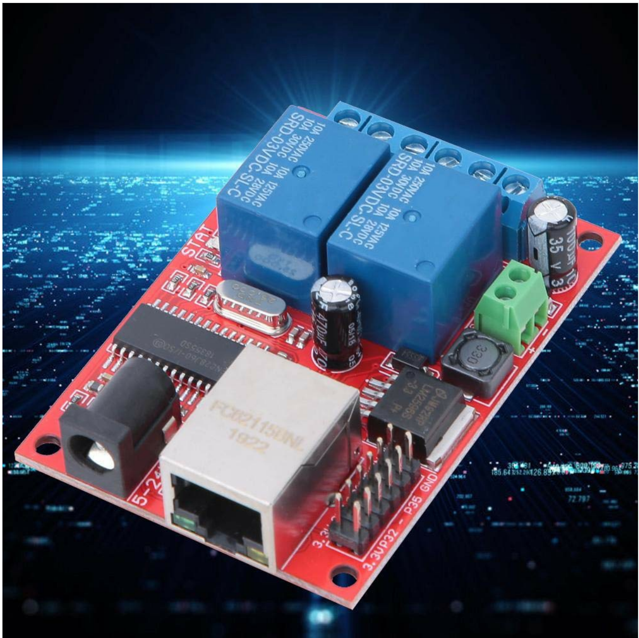
Figure 2: Angled view showing the LAN port and power input.
