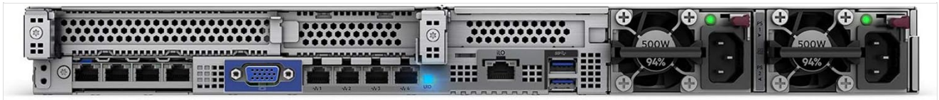
Figure 2: Rear view of the server, highlighting power supply units and network interfaces.
