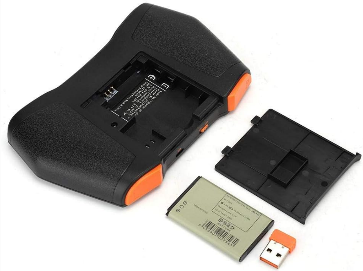
Image 3.1: Location of the USB receiver and battery compartment.
