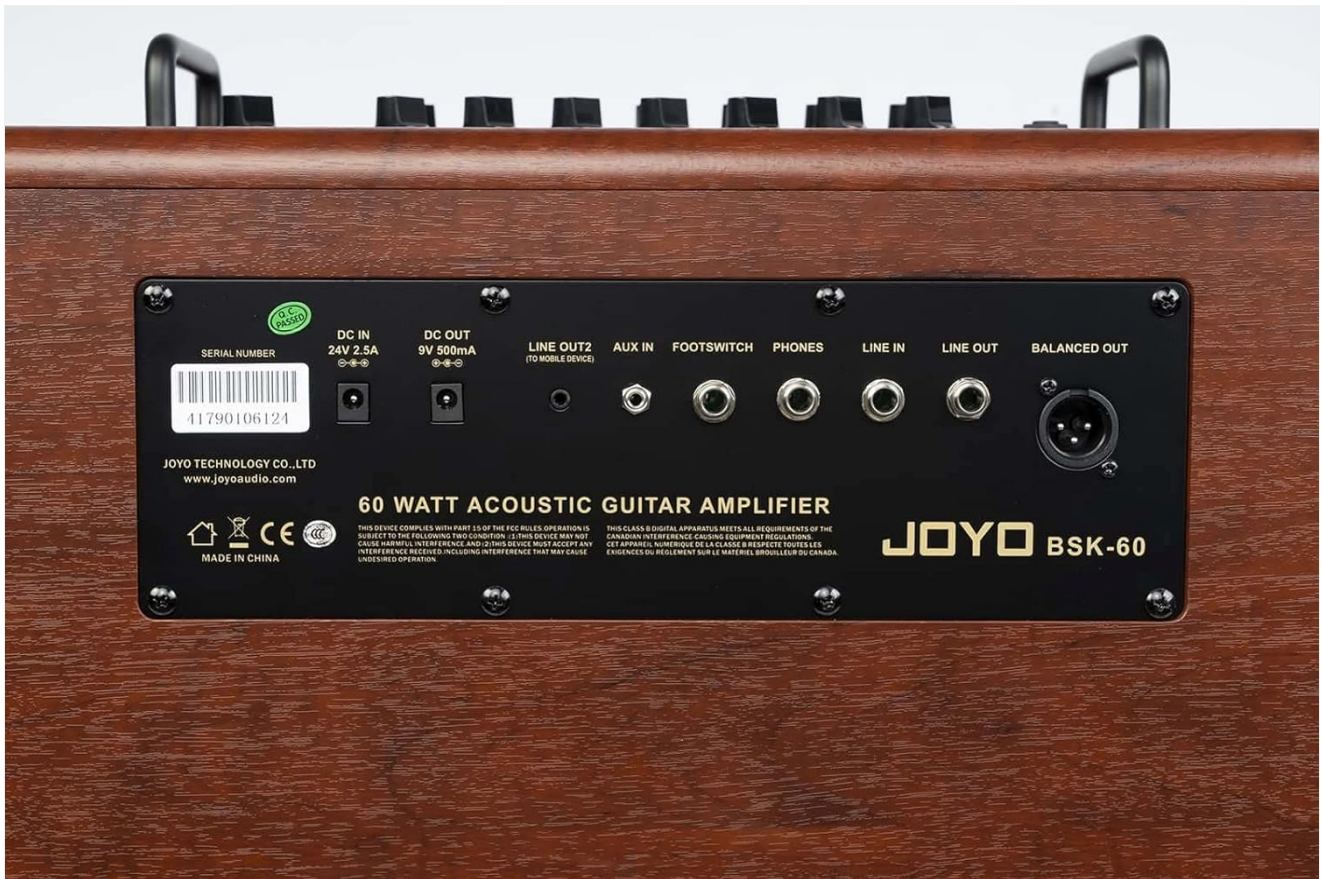
Figure 4.4: Rear panel of the amplifier, displaying various input/output ports such as DC IN, DC OUT, AUX IN, Footswitch, Phones, Line IN/OUT, and Balanced OUT.
