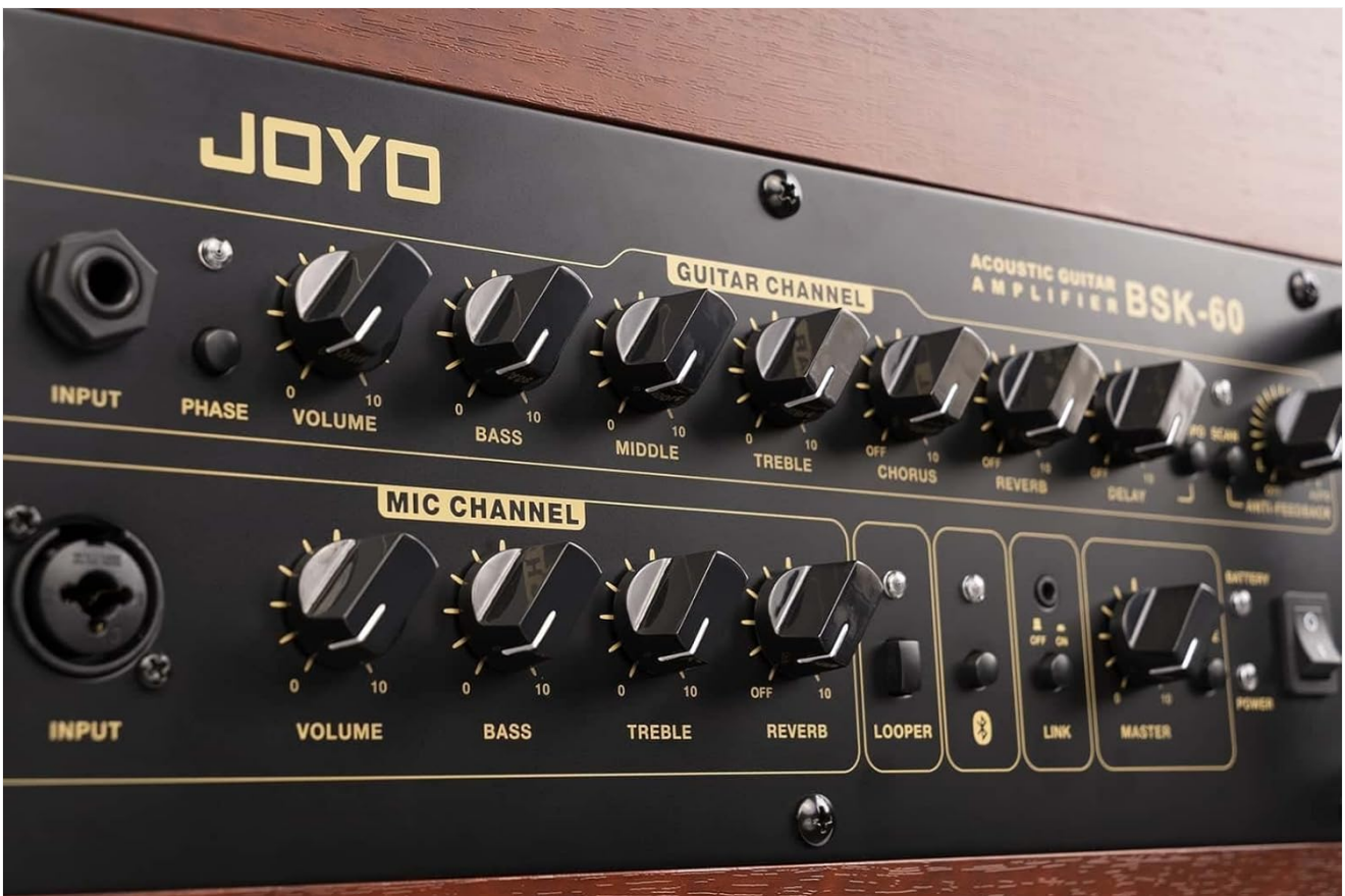
Figure 4.3: Close-up of the control panel, showing Guitar Channel and Mic Channel controls, including input jacks, volume, EQ, and effects.
