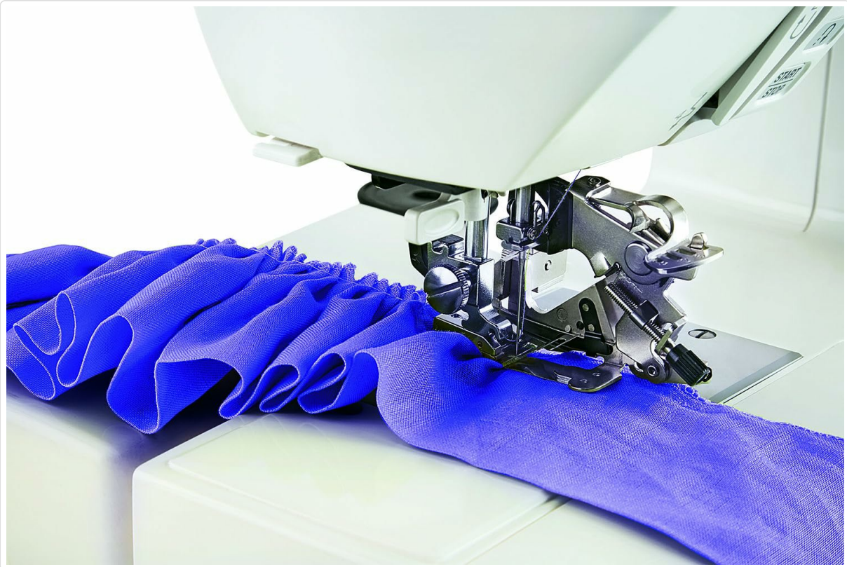
Image: The Usha Janome Marvela sewing machine demonstrating the ruffling application on a blue fabric.
