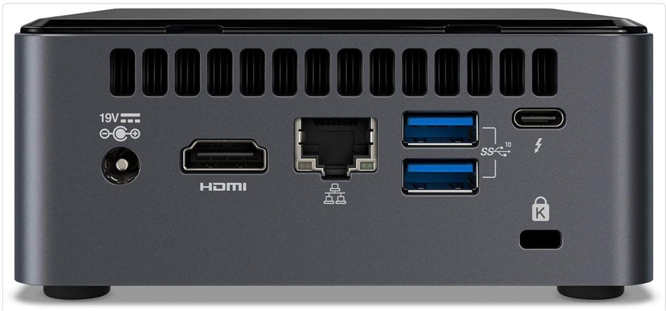
Image: A detailed view of the rear ports on the Intel NUC 10, including power, HDMI, Ethernet, USB, and Thunderbolt 3.
