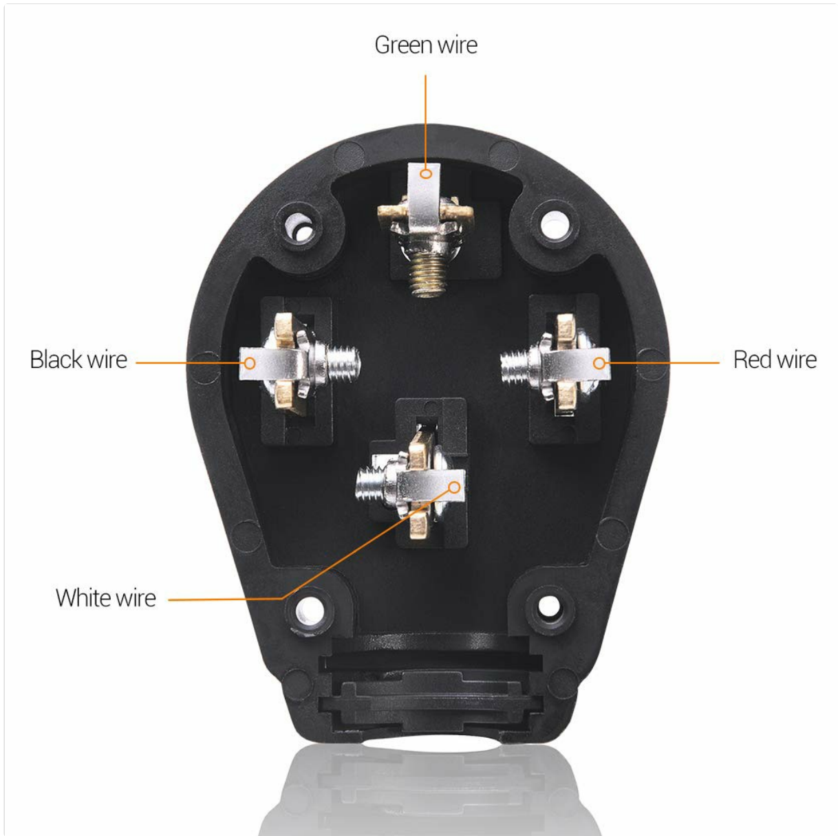
Image 4.1: Internal view of the Nema 14-50P plug, indicating the connection points for the Green (Ground), Black (Hot), Red (Hot), and White (Neutral) wires.
