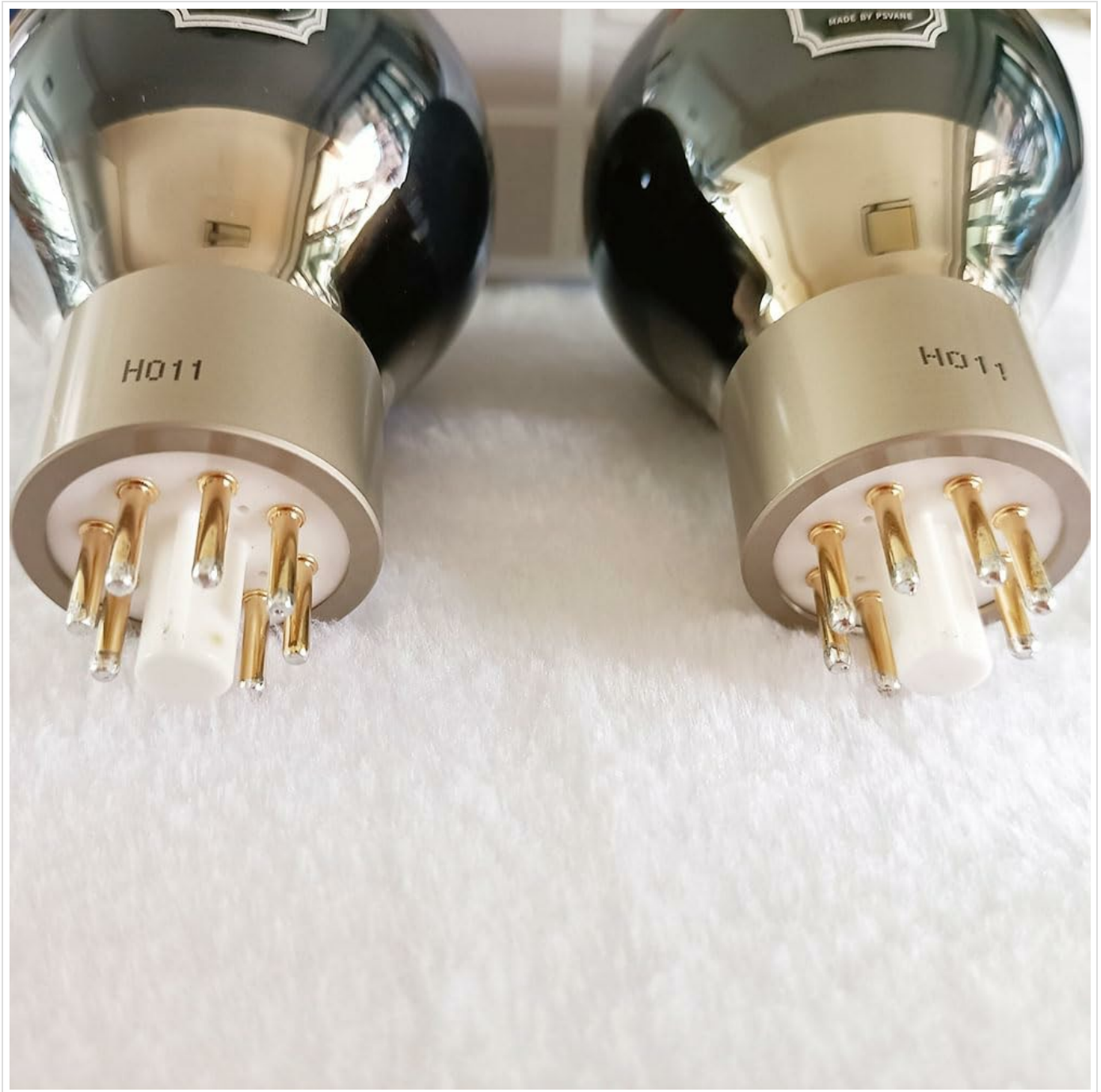
Image: A detailed view of the base and pins of a PSVANE Cossor 6SN7 vacuum tube, illustrating the robust construction and pin configuration essential for proper insertion into an amplifier socket.
