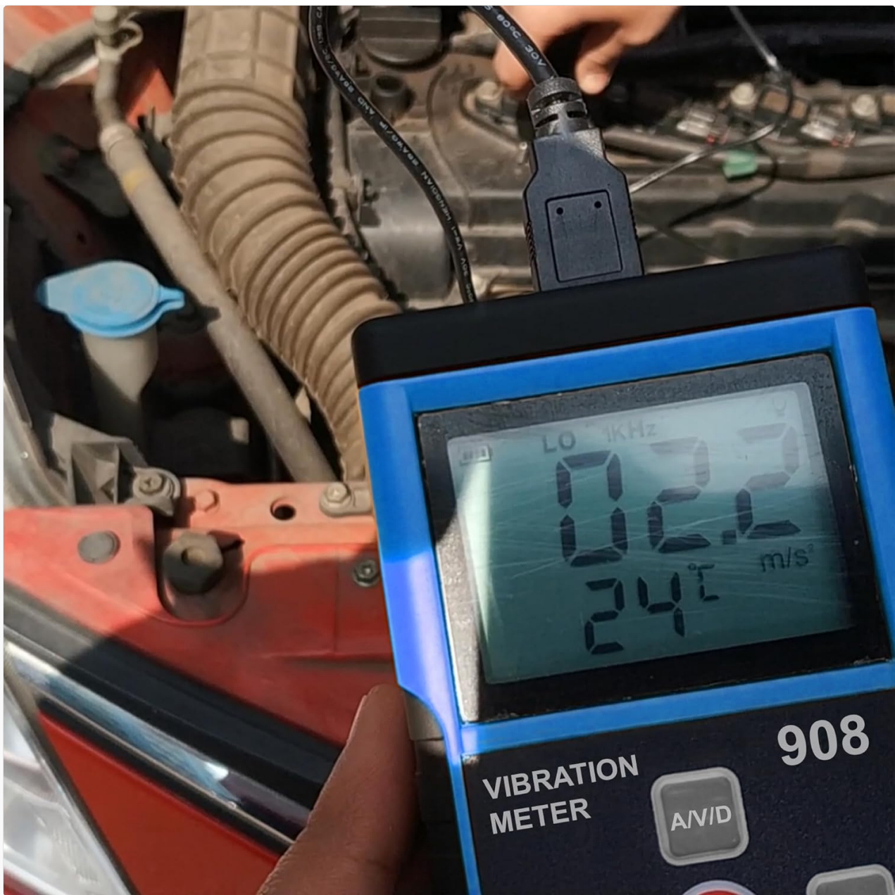
A detailed view of the Metravi 908 Vibration Meter's LCD display, showing active measurement readings for vibration and temperature, with the probe connected to an object.
