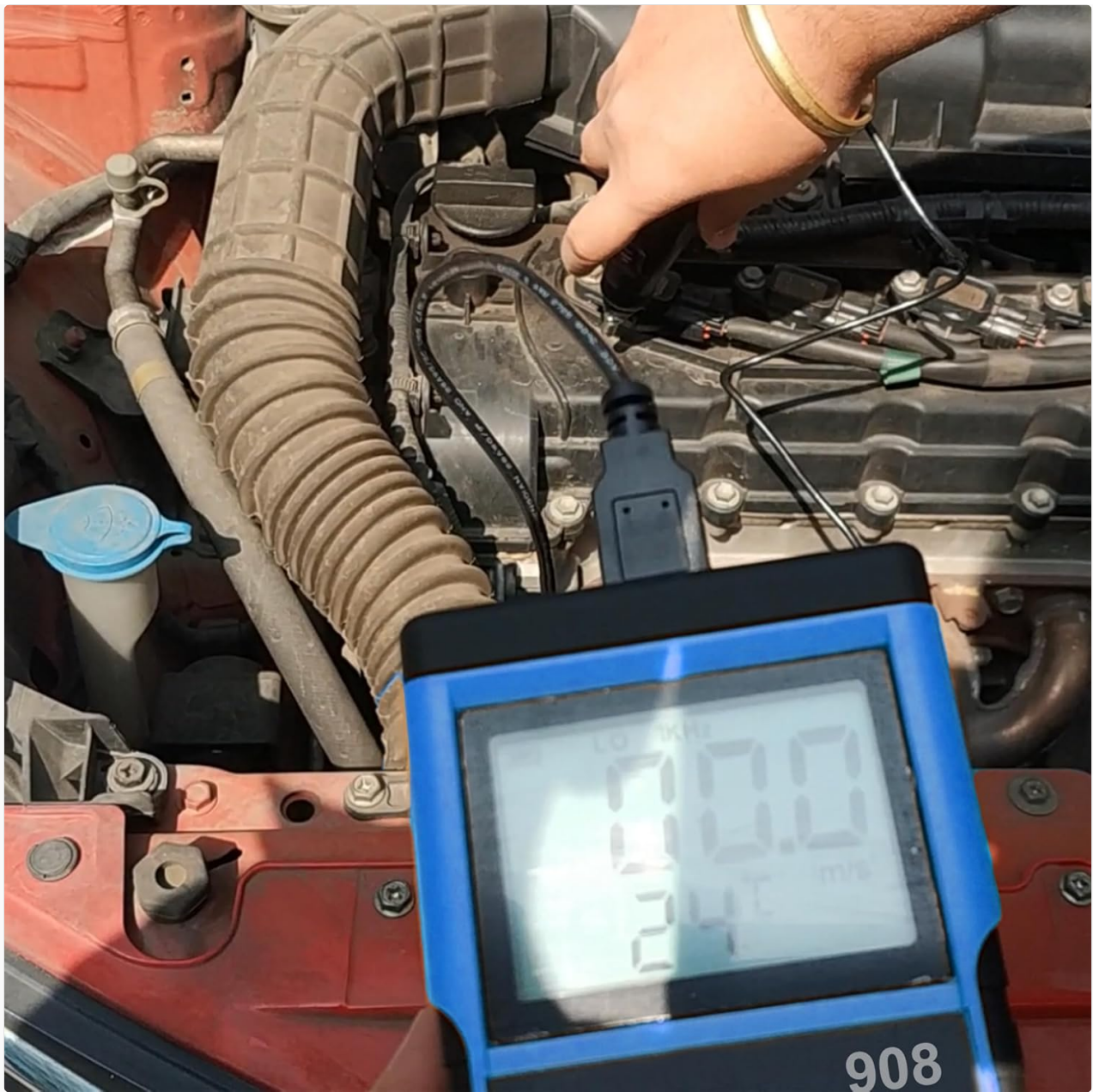
The Metravi 908 Vibration Meter in operation, with its probe attached to a vehicle engine to measure vibrations. The meter's display shows current readings.
