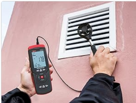
Figure 4: Measuring air volume from a ventilation outlet.
