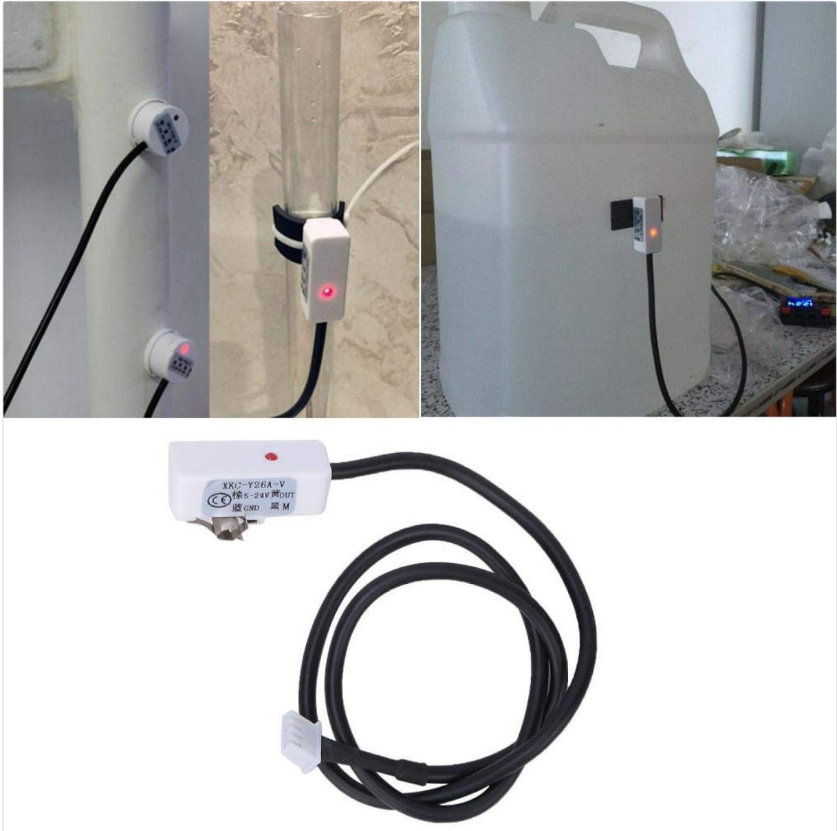
Image 6.1: Application Examples. This image collage demonstrates the sensor's use in different scenarios, including attachment to a large plastic container, a clear pipe, and a smaller bottle, showcasing its adaptability for various non-metallic liquid containers.
