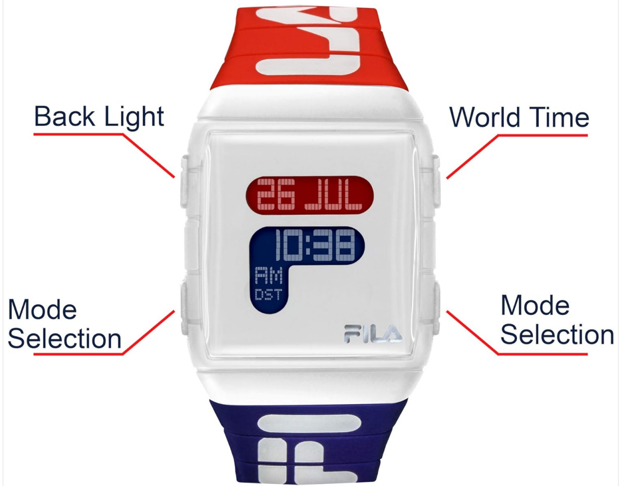
Figure 3: Watch Components and Button Functions
